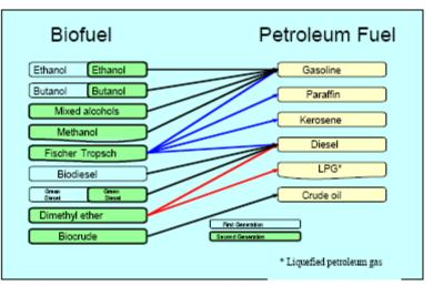
Fig. 1. Substitutability of biofuels with common petroleum-derived fuels.
