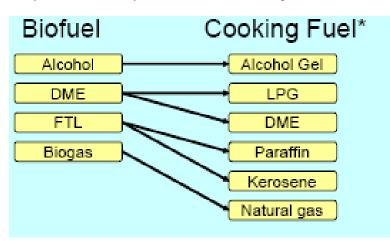
Fig. 2. Substitutability of biofuels for clean fossil fuels used for cooking.
